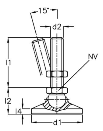
A/F = 12 d1 = 25 d2 = 8 l1 = 63 l2 = l4 = -Static load (N) = 7 Weight in (g) = 67
